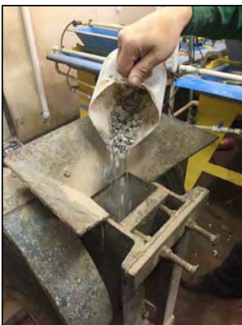
Oro ore in the jaw crusher
