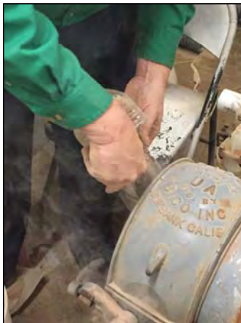
Oro ore being pulverized
