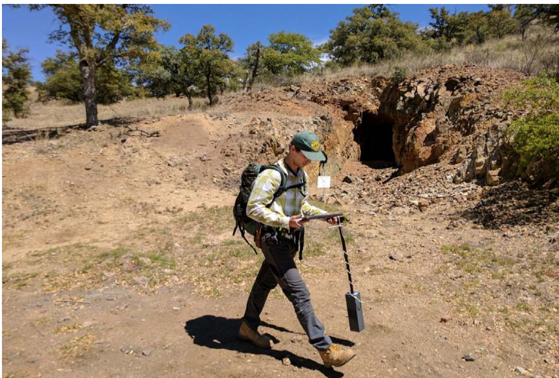
Running Hand Held Electro Magnetic Pin Pointer To Look For Mineral Concentrations
